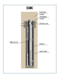
Filled with fuel combat missile is kept in a hermetically sealed transporting and launching canister (TLC) with folded wings and fins. The scheduled check-ups are performed without taking a missile out of the launcher.
